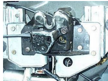
Manual hatch release Figure 2
