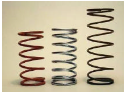
VAFPR spring on left, p/n 105290 center, non-adjust FPR spring on right
